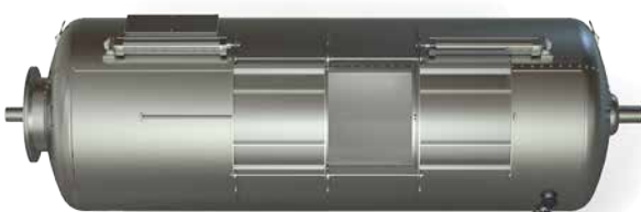
sliding hatch (two leaves) pneumatic drive
