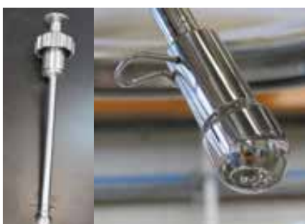
CIP lance with rotating spray ball
