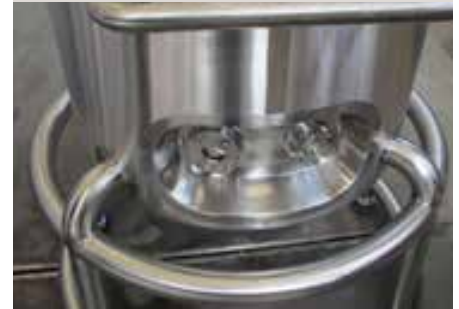
removable lid with hinged screw clamps
